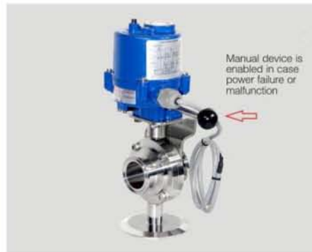
Electric butterfly valve AC 220/110V DC 24V Functions: on/off, intelligent, position sensor Manual device is enabled in case power failure or malfunction
